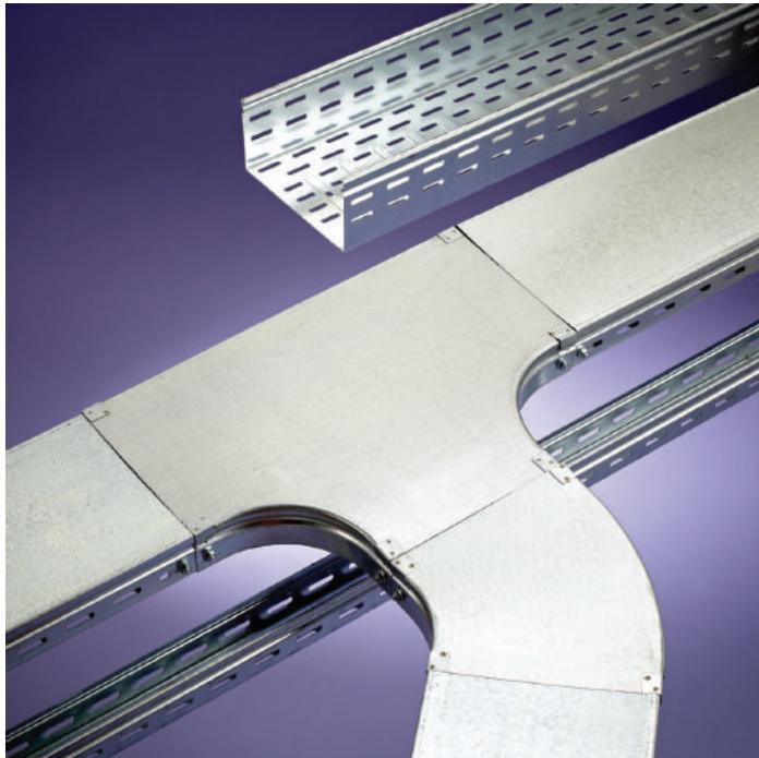
**Ventilated Design** All V-Trough straight sections are ventilated to reduce cable bundle heating, and to keep mold and moisture from building up within the cable pathway.
