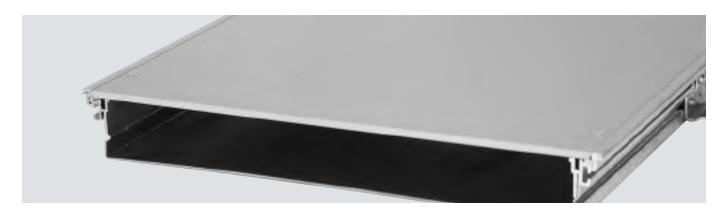
Trenchduct allows easy access to cabling after installation via removable cover plates. It features extremely large cable capacity and is available in many different widths and depths to accommodate all jobs. Trenchduct is installed above the Walkerduct or Walkercell system, flush with the finished floor.
