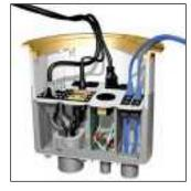
Internal wiring capacity. Evolution Series 10" pokethru devices are the first in the industry with the capacity to accommodate wiring connections inside the unit, eliminating the need for an external junction box and making future moves, adds and changes faster and easier.
