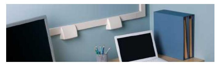
Dual channel version of 2400 Series Raceway. Easy-to-install and ideal for basic power and communication/low voltage installations in classrooms, hotels, and anywhere a low profile raceway solution is needed.
