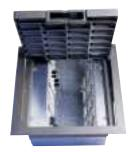
The AC10105-2 box with a 5" (127mm) depth is a square profile box that provides eight-gangs of power and/or communication device capacity. Power plate with duplex knockouts included with box. The AC10105-2 also provides increased plug-in volume which is ideal for the additional space needed when plugging in transformer type plugs. Lids can be rotated 180° for easy orientation. Gray lids are die-cast zinc construction.
