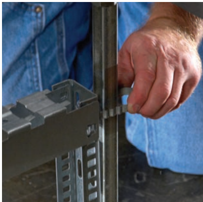
Place assembly leg supports in position and loosely secure to floor legs with serrated attachment clips.
